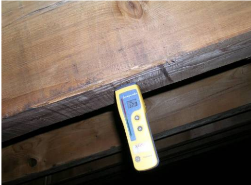
Figure 16. Humidity reading with electric xilohigrometer.
