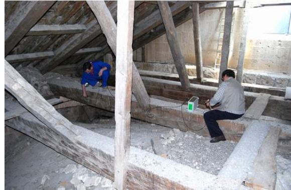
Figure 17. Measuring ultrasonic speed.
