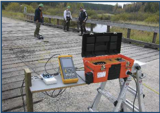
Figure 9. — Testing a timber bridge using vibration techniques.
