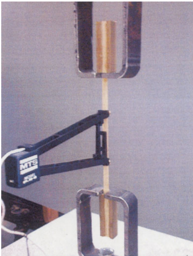
Fig. 13 Testing of the tensile micro-specimen. The central portion defining the gauge length is machined to a smaller cross-section
